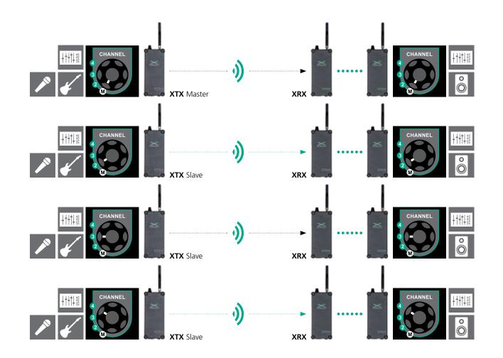
The system may be expanded to four sound channels for the transmission of several, different audio respectively stereo signals. For this purpose one of the XTX transmitters with the first audio channel assumes the role of the master, to which one may connect three more XTX transmitters that facilitate the transmission of the other audio channels. This set up also allows the use of a limitless number of XRX receivers, which can selectively receive one of the four audio channels.
