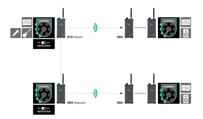
The XRX can either be used as a receiver or as a repeater. In repeater mode the XRX forwards the audio signal received from the XTX without any changes, which in turn can now be received by an unlimited number of XRX receivers set to reception mode. The repeater represents the perfect addition to the system: it doubles the range of the system and helps to overcome walls, corners or other obstacles. In repeater mode the XRX transmits either two audio signals or one stereo signal.
