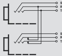
This is the most common configuration, very often called HALF NORMALLED. In this configuration internal normalling contacts connect the top jack contact with the corresponding bottom jack contact. Inserting a plug in the bottom jack will
