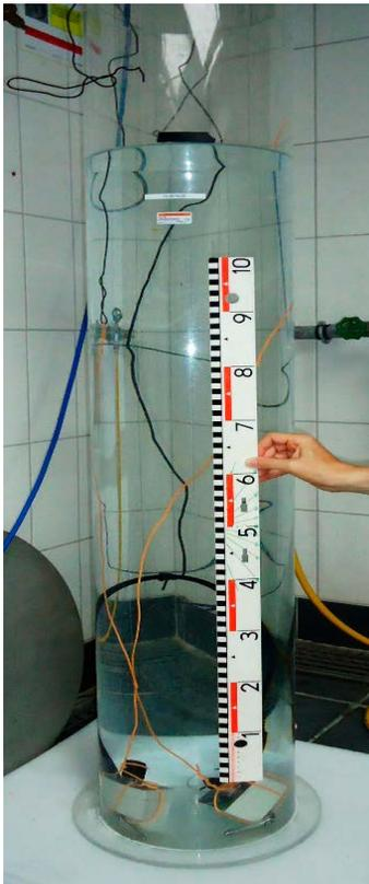
Table 13.a: NO2MW-XP and NO2FW-XP immersion by 1.2 m for 30 min.
