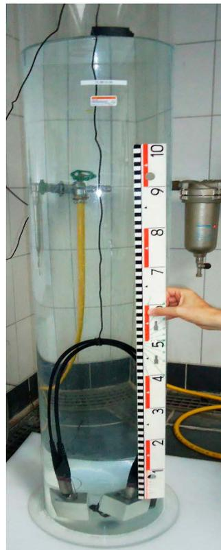
Table 13.b: Connected DRAGONFLY System immersion by 1.2 m for 30 min.
