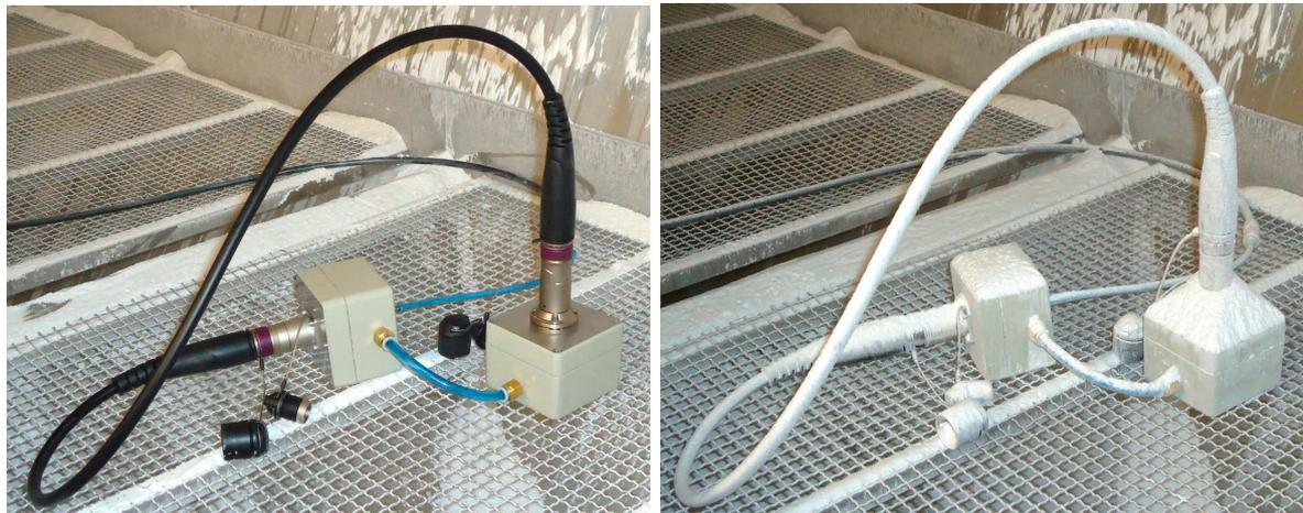
Table 12.b: Connected DRAGONFLY System before and after the dust chamber.
