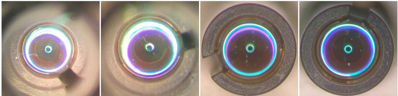
figure 7.d: Lens condition after 10.000 cycles
