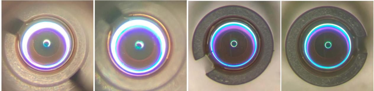
figure 7.c: Lens condition after 3.800 cycles
