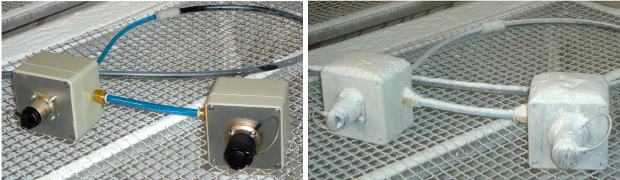
Table 12.a: NO2MW-XP and NO2FW-XP before and after the dust chamber.
