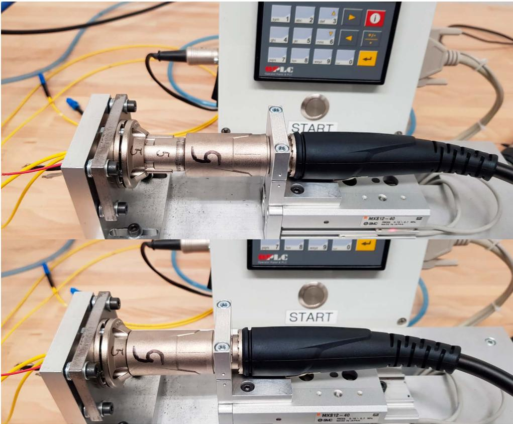
figure 7.b: fixture for 10.000 mating cycles
