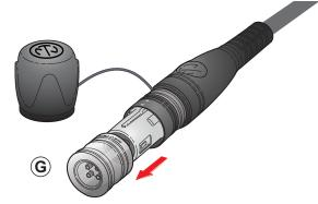
**1.9** After the cleaning procedure unlock the NEUTRIK inspection tool (G).
