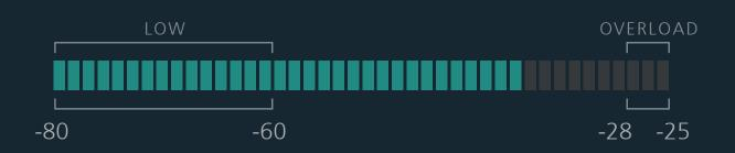
Good signal quality is not only measured by having the highest RSSI level. It's more important to have low packet loss (i.e. green bars). When necessary, engage the RX -30 dB attenuater in the app by setting it to ON.
