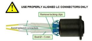
Avoid splayed connectors by using LCs without anti-snag collars and a boot diameter < 5 mm (available from suppliers as e.g. Corning).
