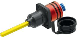
Benefiting from the expanded beam technology and the precision optical alignment the system creates high immunity against dust, mud, liquids and other contaminations. The FIBERFOX EBC15 2CH fixed patch cable connector converts a standardized LC patch cable into an expanded beam solution. It acts as a "feed-through".
